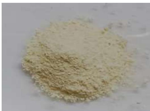
**Figure 1** Green synthesized tin(IV) oxide nanoparticles
