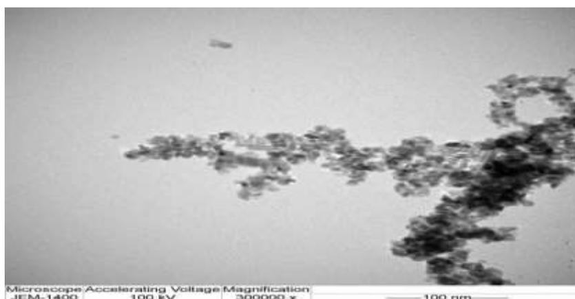
**Figure 6** TEM image of SnO<sub>2</sub> NPs using aqueous peels extract of lime
